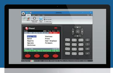
**OMNIPANEL®** is another feature that makes the OMNI 4000/7000 user friendly. OMNI-PANEL is a convenient, Windows-based software application that delivers the look and function of the OMNI 4000/7000 front panel via a software interface.
